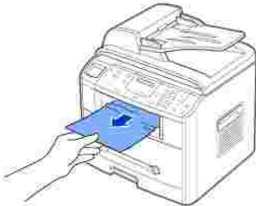
3. *If you cannot see the paper in the front output tray or the paper does not move when pulled, open the rear cover.*
